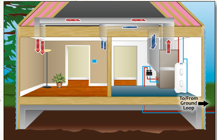
The above illustration depicts a typical packaged system installation with forced air in heating mode. Other installation options are possible.
