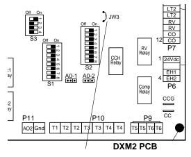
JW3-LT1 jumper should be clipped for low temperature (antifreeze) operation
