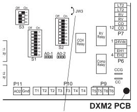
JW3-LT1 jumper should be clipped for low temperature operation
