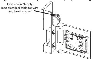
Figure 23: Outdoor Compressor Section (TEP) Line Voltage Field Wiring
