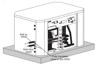
Figure 21d: HWG Service Valves
