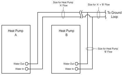
When the number of units or flushing requirements reaches a point where it is no longer feasible to flush through the internal valves (generally systems of more than 12 tons depending on loop design), external flushing valves should be installed. In this case, three-way flushing valves should be used or additional isolation valves must be installed to be able to isolate the loop during flushing.
