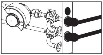
Flow rates between 2.25 and 3 gpm per ton [2.41 to 3.23 l/m per kW] of cooling capacity is recommended in these applications.
