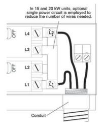
Figure 16: Power Wiring, 4, 5, 8, and 10kw
