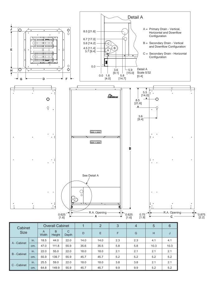
The Tranquility Air Handlers are designed for upflow, horizontal, and downflow applications. The coils have a dry nitrogen holding charge and are equipped with brazing stub refrigerant connections for easy installation. Both models come equipped with a factory installed TXV.
