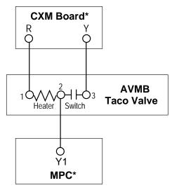
\*Valve must be wired in between the CXM and MPC boards. Remove the yellow wire from the CXM board and connect it to terminal 2 on the valve. Add a new wire from terminal 3 to the Y terminal at the CXM board, and a jumper wire from terminal 1 to terminal R at the CXM board as shown above.
